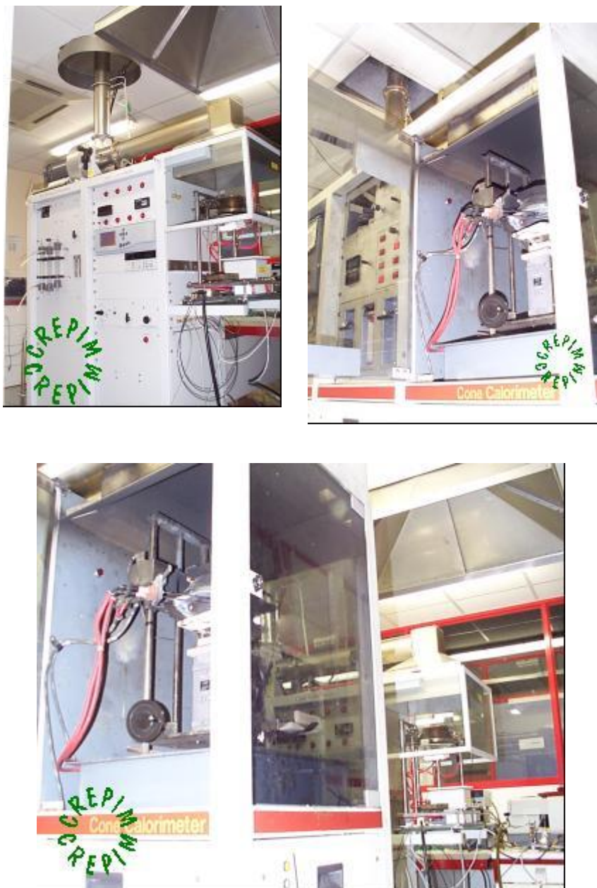
Figure 12: The ISO 5660 cone calorimeter test method
